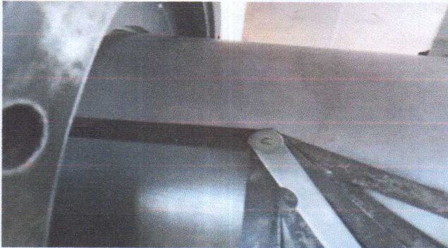
Clearance Check Shaft Propeller
