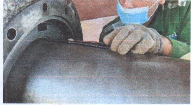
Clearance Check Shaft Propeller
