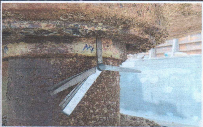
Clearance Check Rudder Stock
