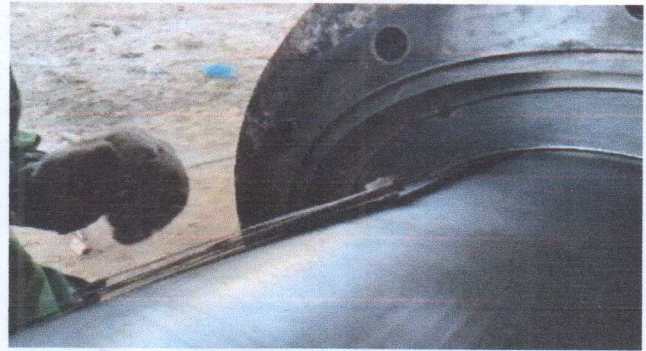
Clearance Check Shaft Propeller
